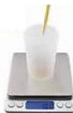
Weigh out approx. 1000g of sample. Add distilled water<sup>1</sup> until the total desired weight (dilution ratio)<sup>2</sup> is reached. Stir well.
