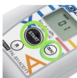
Use the START and ZERO buttons to select the desired scale.
