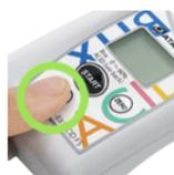
Press and hold the Brix-Acid Ratio button until the scale selection screen is displayed (after 5 seconds).
