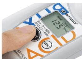
Press START. Brix result will be displayed. Be sure to thoroughly clean and wipe off the sample stage after taking measurements.
