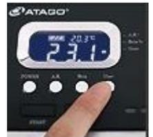
**Point 4 - Measurement evaluation indicator** - Measurements are evaluated against pre-set tolerance limits, and the result is indicated by green or red light. (Upper and lower tolerance limits must be set in advance to using this function)
